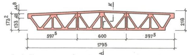
Figure 3 – Illustration of prestressed truss, in m.
