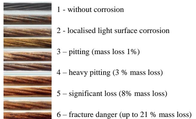
Figure 4 - Illustration of grades of reinforcement corrosion
